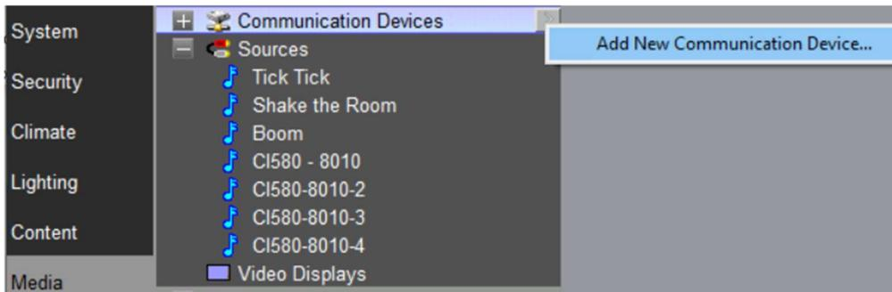
Select “BluOS Media Comm” driver to install. Once it’s installed, it will start to discover all BluOS players on the network automatically. A set of Media Renderer driver and Zone Controller driver for each player will be automatically installed. Please note that the discovery will be disabled automatically after 10 minutes. Click “Discovery Players” again to initiate the player discovery again.
