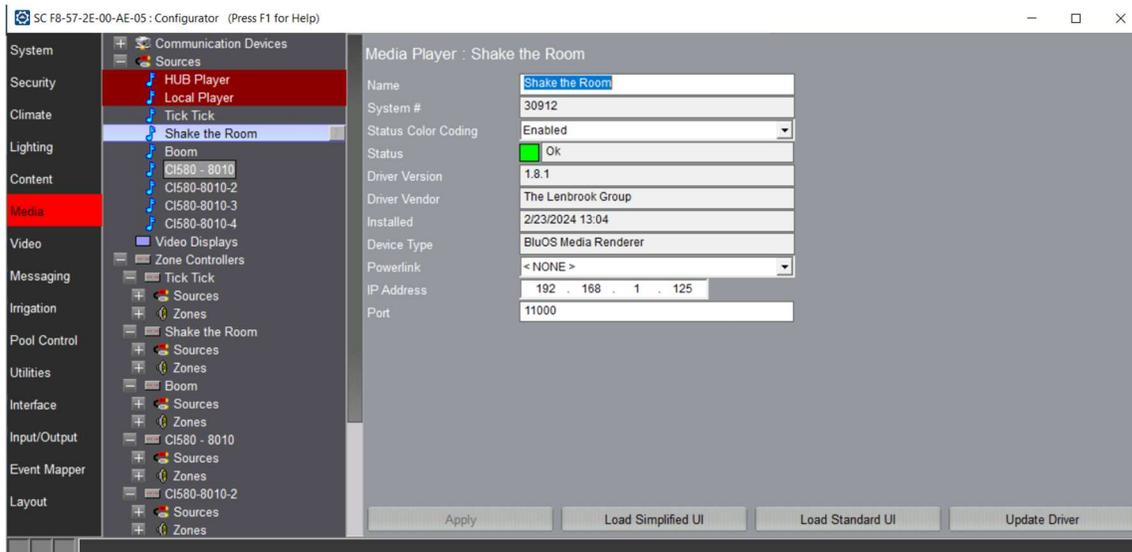
The Media Renderer also provides commands to load Simplified and Standard UI for event programming.
